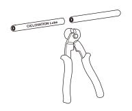
3. After cutting, use the cable cutter to correct the distortion of the outer casing. And install end caps.
